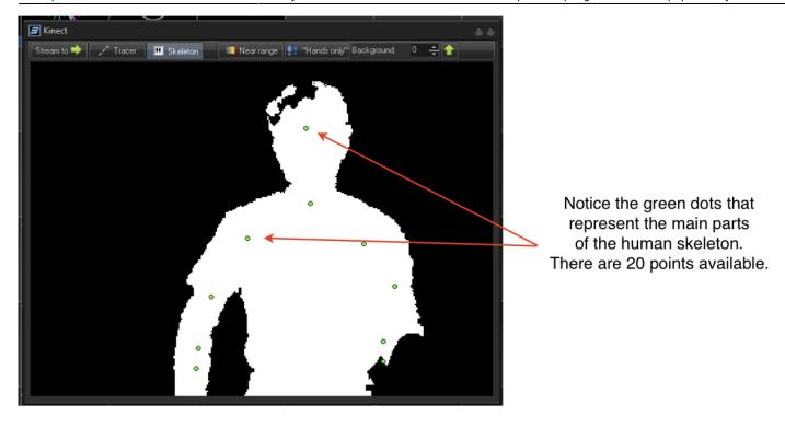
There are 20 points in the skeleton. Each point has X, Y, Z coordinates and an activity flag. If the point is not visible (meaning it can not be recognized by the Kinect) than the value of the active property is zero. If the point is visible, than the value of the active property is one.
