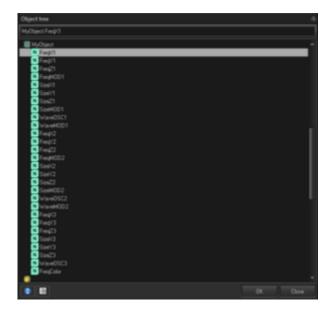
Public objects can be controlled by means of Universe components such as a slider. The Slider component has a "Link to" property what will allow it to create bidirectional links between the Abstract object and the slider. On the screenshot panel within the Universe Inspector, click on "..." call Object Tree dialog, where you can select the object from the Object Tree (screenshot below).
