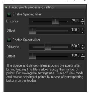
The **Spacing** and **Smooth** filters allows you to reduce the number of output points. Minimum values give "soft" effects. Values closer to maximum give the maximum effect. Do not forget to enable "Show point" if you want to see the result of filters on the PC monitor.
