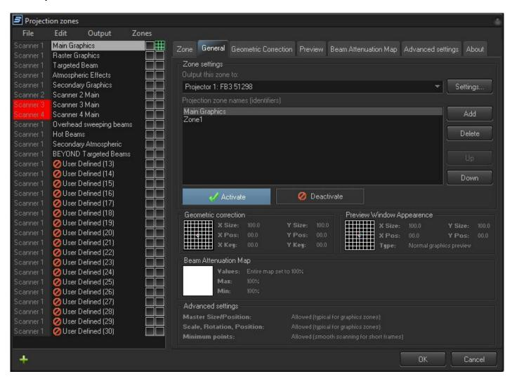
The list of projection zones can be seen and selected on the left side of the window. When you click on a zone in the left side, the tabs on the right allow you to view and adjust the parameters for each projection zone. To view and adjust the parameters, click on the Geometric Correction, Preview Window Appearance, Beam Attenuation Map or Other tab.
