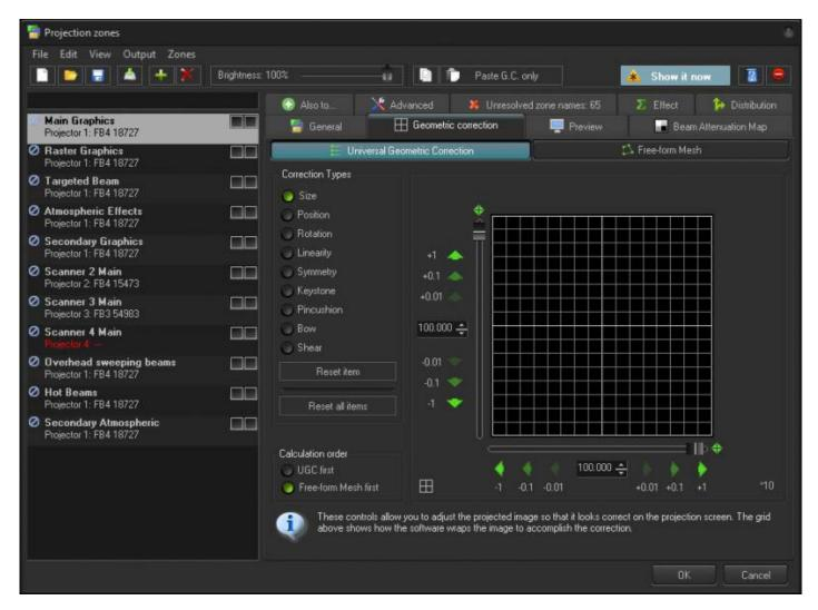
To adjust the geometric correction in BEYOND, you have two options. First, you can use the Universal Geometric correction tools (similar to QuickShow and LD2000) or you can use the Free-form Mesh tool, or you can use both.
