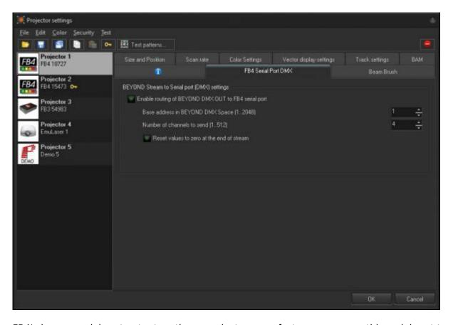
FB4's have a serial port output on them, projector manufacturers may use this serial port to output data inside the projector, or even through the FB4 dmx output (if wired). This allows you to control internal systems like grating wheels and drop in filters, or output a dmx stream from the FB4. If wired, you can add "serial\_mode=4" to the INI file to use it as a dmx output node, however it will no longer function as a DMX in, only output.
