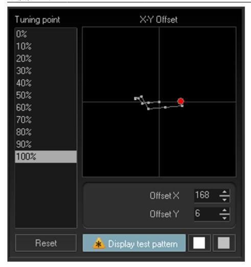
Beam Brush® systems as they move through brush values will create a slight X-Y shift in output. This can be minimized with perfect alignment, but in the reality of the touring world, this is unachievable, so we have added a X-Y compensation to tune this shift and make your output perfectly smooth. This X-Y offset is done before the output scaling and Linearity correction This means that it counts for the full 100% of the potential brush range. So, scaling afterwards will not affect X-Y Offset.
