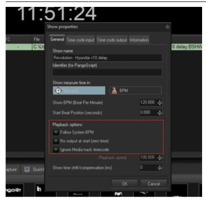
Follow System BPM - Overwrites show BPM and forces usage of BPM from the Grid mode toolbar (main system BPM) No Output at start. Only when a show is driven by timecode, and is waiting on position 0, do not generate output to laser, even if show events starts from position 0.
