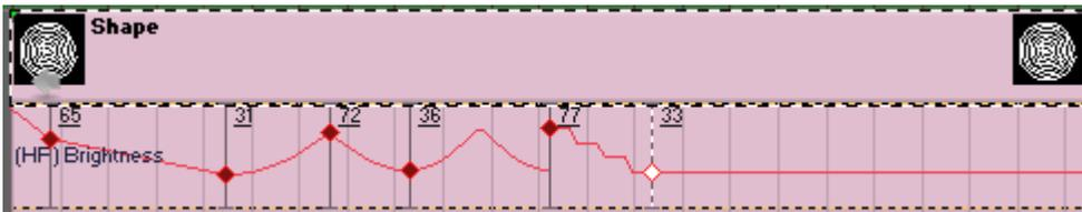
The small nodes can be moved up and down which will change the value. The rate of change (acceleration) is controlled by the context menu of the key. The context menu is available by right clicking on the key-icon in the TimeLine as well as in the Effect tab.
