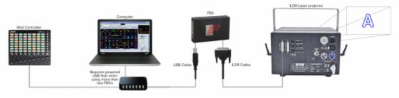
NEX CONTROL SETUP Here you can see a basic witup including an AFCMIN midl console using a single later projector. The same principles for shared and independent control, mentioned above, apply here
