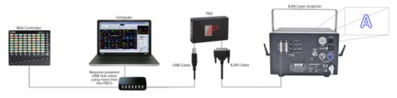
MEX CONTROL SETUP Here you can see a basic setup including on APCMIN mill console using a single laser projector. The same principles for shared and independent control, mentioned above, apply here
