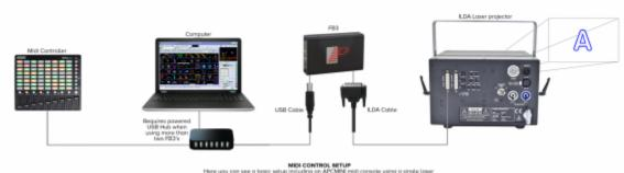
Here you can see a basic setup including an APCMM midl console using a single lawer rejector. The same principles for shared and independent control mentioned above, apply here
