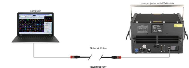
In this setup we have a single laser projector connected to our PC via the Integrated FB4 hardware.
