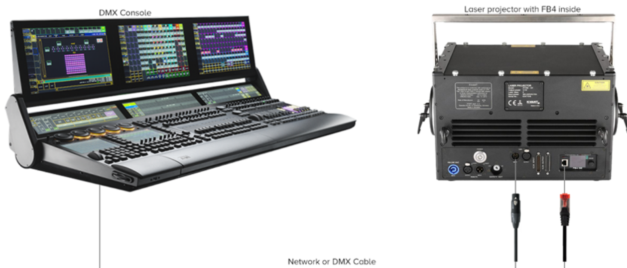
CONSOLE SETUP In this setup we have a single laser projector connected to a dmx console via the integrated FB4 oem hardware through DMX or Ethernet. This example requires the FB4 DMX or FB4 MAX. The FB4 has been pre-populated with frames and can operate without computer.
