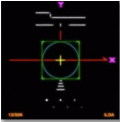
Scanning correctly: Circle touches midpoint of square
