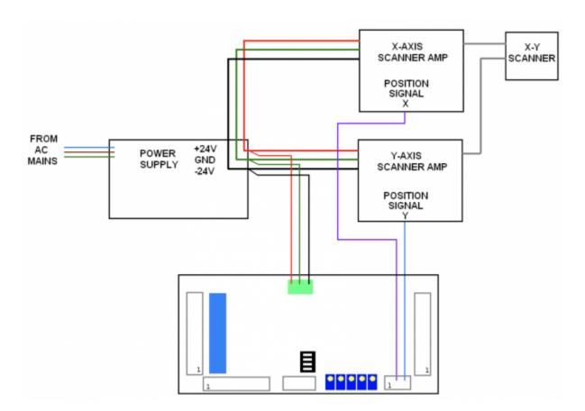
PASS monitors the power supplies that feed the scanner amplifiers. This voltage can be between  $\pm$ 0 volts and  $\pm$ 1 volts. The manner in which you connect PASS to the power supply and to the scanner amplifiers depends heavily upon whether you are using two separate single-axis scanner amplifiers, or one dual-axis scanner amplifier.
