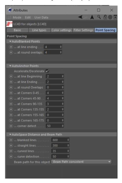
**Note**: The numbers shown above are the default values. They are optimized for scanners tuned to the ILDA 30K standard, when running at a point output speed of 30,000 points per second. If you do not change any of the numbers, objects will use the default values. For more information, see the topic Scan speeds and LC 4D.
