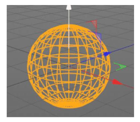
Note that since the mesh polygons are actually triangular, there are many more edges that make up this sphere, but the additional edges are not displayed in the edge selection mode. If all edges would be visible, the sphere looks like this:
