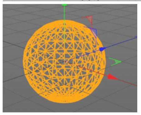
Normally, you would use the Edge Selection line type to easily and quickly create a geometric, or high-tech look of the object. But in addition to simple geometric looks, you can use Cinema 4D's ability to designate certain edges as as an **Edge Selection**, in conjunction with Lasershow Converter 4D's Edge Selection line type to get some interesting results.
