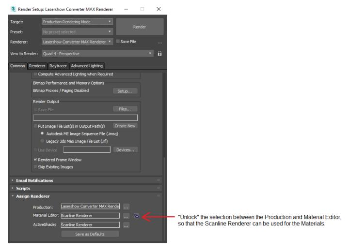
Note: Lasershow Converter MAX can not be used as the ActiveShade renderer.
