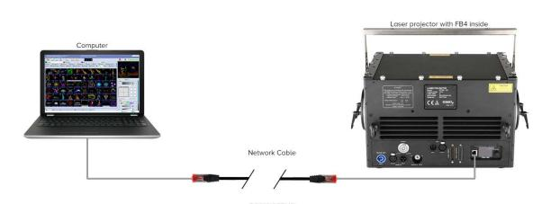
BASIC SETUP In this setup we have a single laser projector connected to our PC via the Integrated FB4 hardware.
