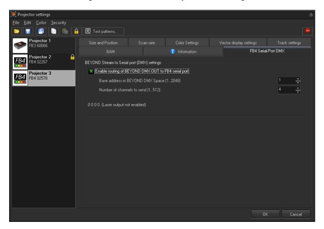
Click the "Enable routing..." checkbox to enable output of DMX through the FB4.
