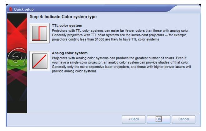
Setup the projector settings and targeted beam positions next
